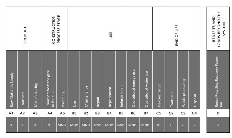
The system boundary covers the production of raw materials, all relevant transport down to factory gate, manufacturing by AGT, deconstruction of the product from its construction site, transport of the deconstructed material to waste processing facility with an assumed distance of 200 km, waste processing and disposal.
